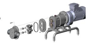
Remove the lobe screws (25) using a wrench that can see on the following figure and it could deliver by Inoxpa. These screws are threaded to the right. Wooden or nylon blocks can be placed between the lobes to stop them from rotation (blocks position: one to the left in front of the top lobe screw and the other to the right in front of the lower lobe screw).
