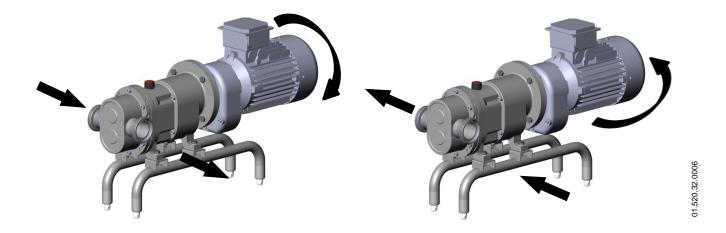
Start and stop the pump motor momentarily. Make sure that the pump rotates in the correctly direction of rotation.
